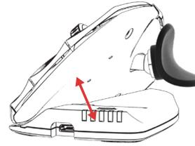
Adjust tilt for your desired mousing angle.
